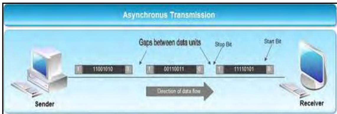
A representation of sender and receiver data transmission in Asynchronous Transmission
