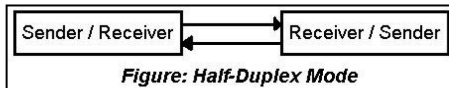
A representation of sender and receiver data transmission in a half-duplex mode
