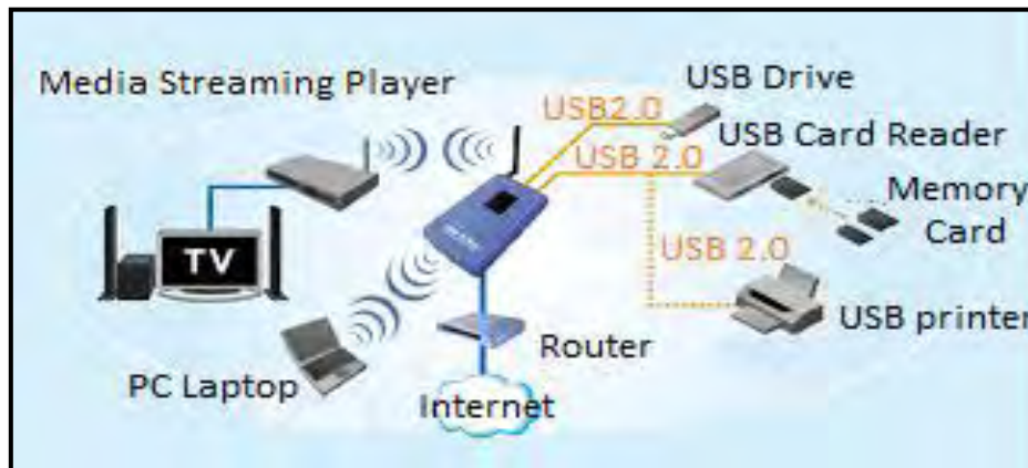
A representation of how devices are linked through wireless communication
